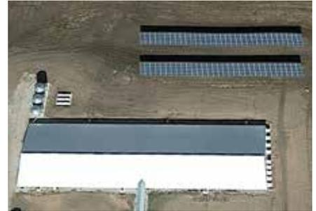
A ground-mounted system situated on the north side of the hog farm, the 117-kilowatt array will produce enough power to nearly eliminate the operation's monthly electric bill.
